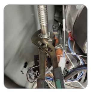
Connect one of the hoses to the outlet of the sump pump and then to the inlet elbow of the heat exchanger.
