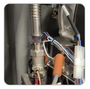
2 Ensure that the drain port is reinstalled with PTFE tape.
