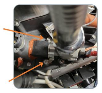
Remove the clip on the inlet elbow by pushing down on both of the tabs.
