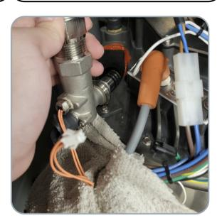
Remove the clip on the inlet elbow by pushing down on both of the tabs.
