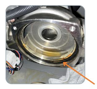
2 Remove the pump cartridge from the silver volute, some water may come out of the pump when removed. Be prepared with some rags as water may drip out.
