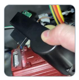
Using the T15 Torx screwdriver, screw in the two screws that hold the bottom of the electrical box to the top of the pump.
