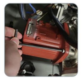
Attach the bottom part of the electrical box to the top of the pump.
