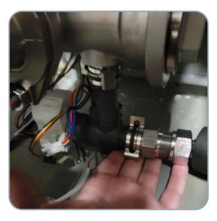
Remove the clip that holds the bottom hex inlet corrugated line and the water valve together. Be prepared with rags as there may be some water left in the lines.
