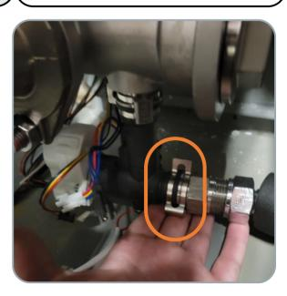
2 Unplug the 3 wire flow sensor harness and the 2 wire inlet temperature sensor harnesses, and move them out of the way.
