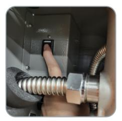
(This forces open all water valves that can open. This will allow the unit to drain completely.)
