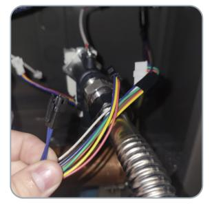
2 Remove the silver clip on the outlet side of the water valve
