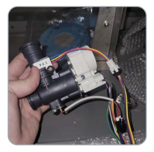
Place the corrugated metal hose inside of the outlet of the water valve, and use the clip to secure it.
