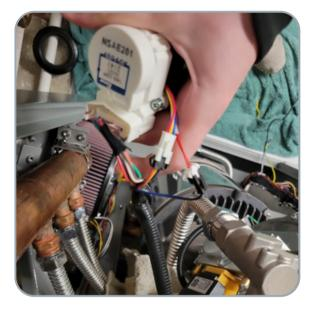
2 Insert the long end of the water valve into the bottom of the top manifold and install the silver clip to hold them together.
