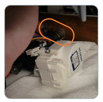
2 Move the 3 wiring harnesses out of the way so if any water comes out when the valve is removed the harnesses do not get wet.
