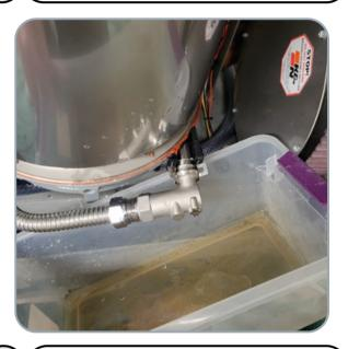
Remove the <sup>3</sup>/<sub>4</sub>" cap on the drain port at the back right on the bottom manifold, near the air filter. With a rag prepared open up the drain port. You will most likely need to close up the port and grab a dry rag, Repeat this process until there is no water left in the manifold.
