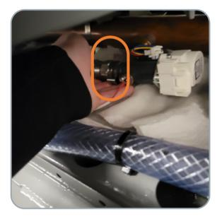
If you replace the O-Rings on either side of the water valve, use Molykote 111 to install the O-Rings.
