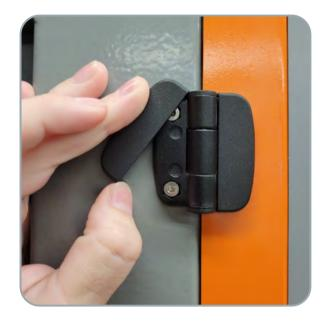
Using a 2.5 mm Allen wrench, remove the screws that hold the hinges to the frame.
