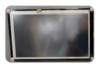
Do not overtighten these nuts as it can interfere with the responsiveness of the display
