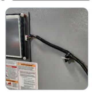
**11** Tighten the zip tie and cut off the excess zip tie.
