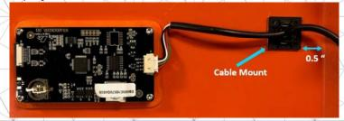
11. Zip tie the other side of the cable with the air switch hose to make sure it doesn't touch the heat exchanger, then power on the unit.
