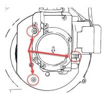
Failure to perform the above change could cause gas leaks. A gas leak check is always required when a gas valve or blower is replaced.
