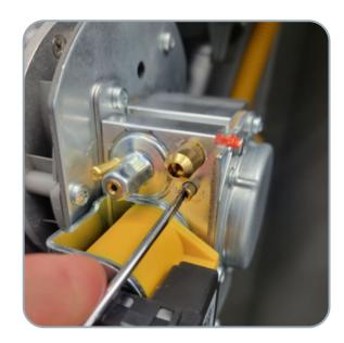
Note: If you are still experiencing combustion rumbling keep increasing the high fire screw by ¼ turn at a time until the combustion rumbling subsides.
