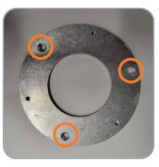
Install the 3 screws that hold the adapter plate to the blower so that they are flush with the adapter plate
