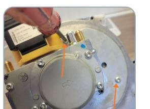
Line the 3 holes that are circled on the adapter 2 plate to the 3 holes circled on the blower
