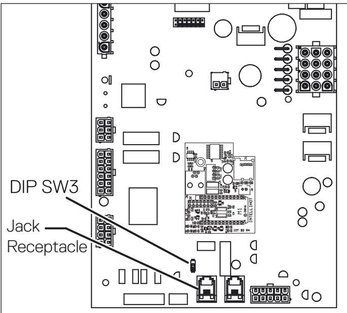
12. Using the supplied cables, connect one end of a cable into either of two jack receptacles (arrows) located on the circuit board and the other end to the jack in the next unit.
