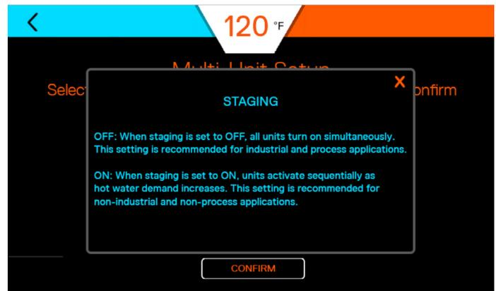
**STAGING ON:** When the staging is set to ON, heat exchangers and units are activated sequentially as hot water demand increases. This setting is recommended for most commercial applications, such as hotels, multi-family, etc.
