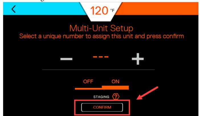
**Note:** Different size water heaters (iQ2001, or iQ3001) can be cascaded together. When assigning unit numbers, start with the smallest unit and progress to the largest.
