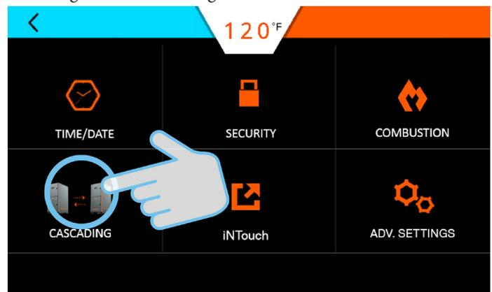
In the Multi-unit Setup, select confirm at the bottom to change the cascading ID.
