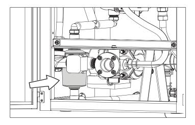
Twist the bottom of the sediment cup to release the locking clips.
