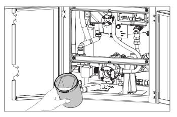
3. Remove the inner sediment cup from inside the lower portion of the unit.
