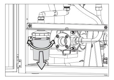
2. Pull down on the sediment cup and pull it away from the upper portion of the unit. The sediment cup will normally be full of condensate. Carefully, pour the condensate into a container and properly dispose of it.
