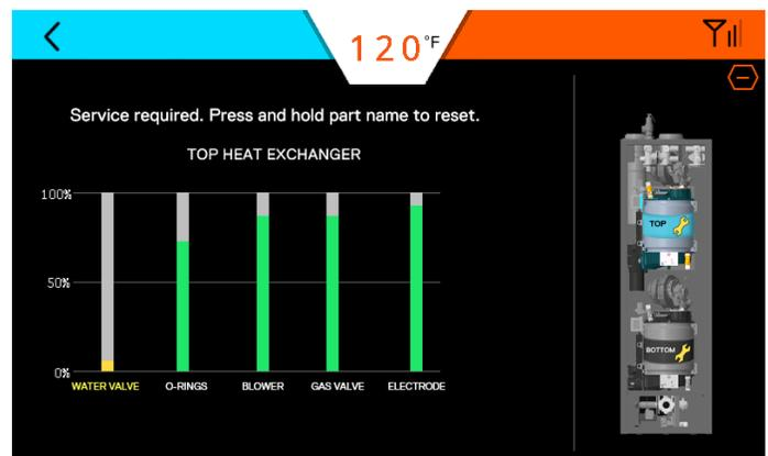
**Service required:** Take IMMEDIATE action when this screen appears because the part life is critical. To reset life, press and hold the appropriate bar and follow the prompts.
