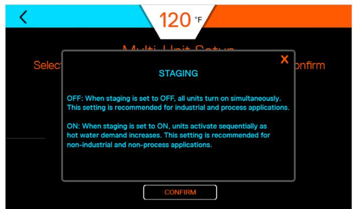
**STAGING ON:** When the staging is set to ON, heat exchangers and units are activated sequentially as hot water demand increases. This setting is recommended for most commercial applications, such as hotels, multi-family, etc.
