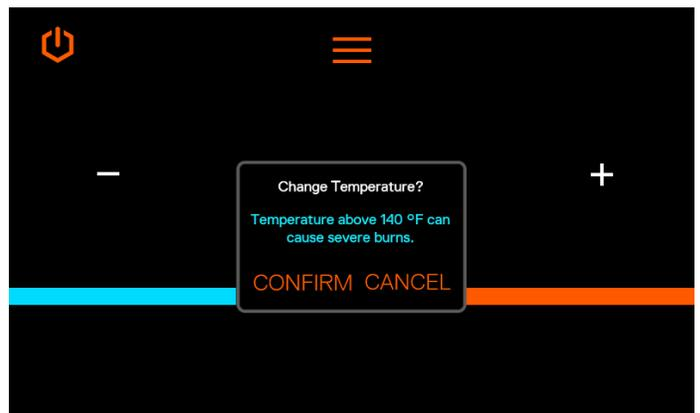
2. For finer temperature adjustments, tap the (+) and (-) icons to change the temperature by 1°F.
