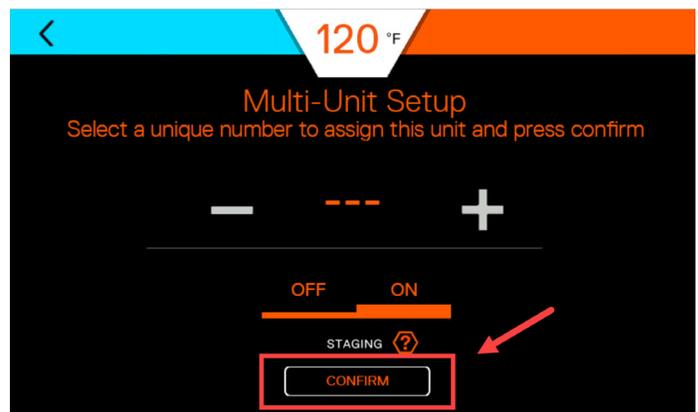
Please ensure the cascading cables between the units (external to the water heaters) are disconnected. This step is critical. After you have verified this, please click Confirm to continue.
