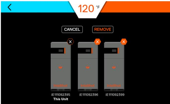
For a cascade setup, click icon above the unit on the screen to add current unit with another available units.
