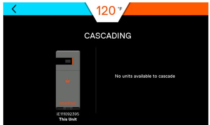
For a cascade setup, click icon above the unit on the screen to add current unit with one available unit.
